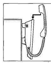
To temporarily set the handset down during a conversation, place it as shown here.
