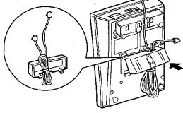
Connect the telephone line cord. Mount the unit, then slide down.
